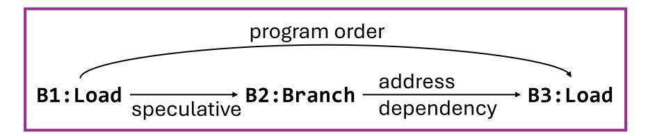
Pattern template (opcode sequence): *w* (1: Load) -- (2: Branch) -- (3: Load)
